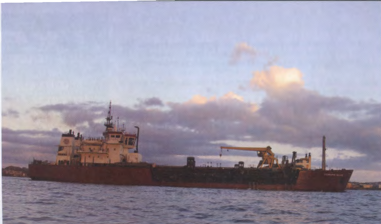
The dredge Terrapin was used to dredge the sand used to cap the Newark Bay CDF. Photo: Linda Guenther, U.S. Army Corps of Engineers
